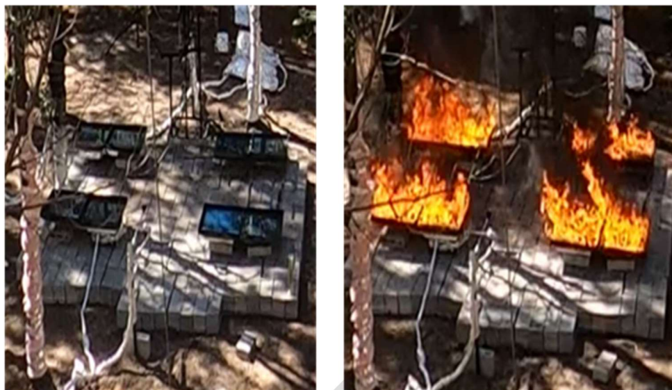
Figure 33. Two rows double-double space (2-2&2-2) – Double line with 4 pans per line with 2-pan spacing between lines and pan sets within each line (Burns 40-41 and 64-65).
