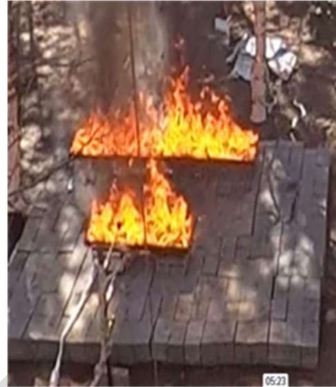
Figure 29. Two rows double space (4&2) Double line with 4 pans in one and 2 in the other with a 2-pan spacing between lines (34-35, 58-59 and 78-79).
