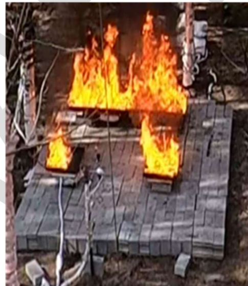
Figure 30. Two rows double-double space (4&1-1) – Double line with 4 pans in one and 2 pans in the other with 2-pan spacing between lines and between 2 pan line (Burns 38-39, and 62-63).
