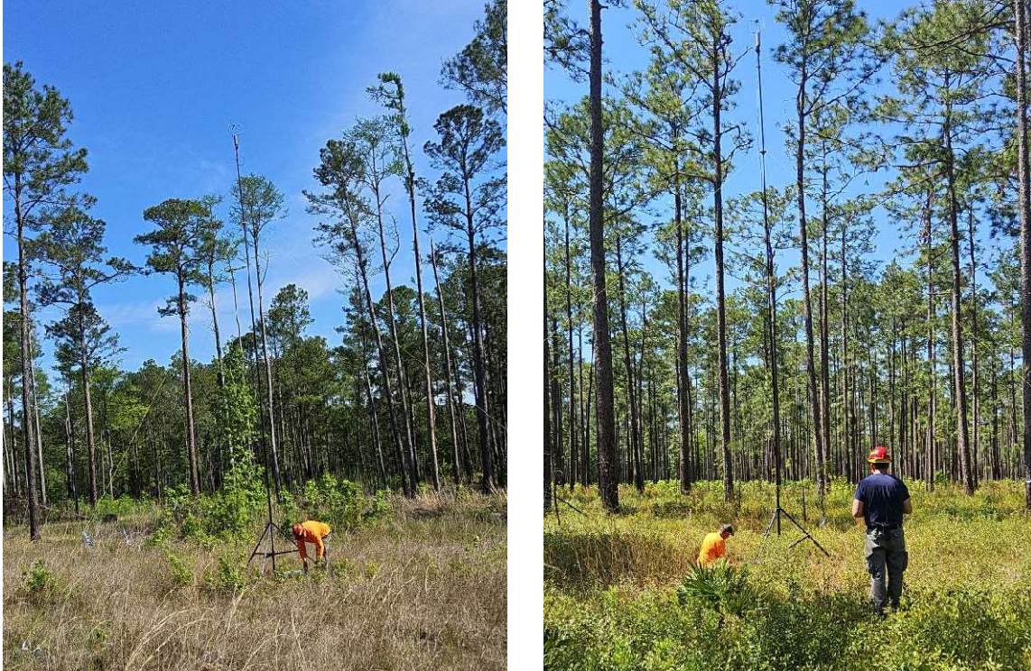
Figure 1. Sonic anemometers set up on the northwest corner (left) and the western edge (right) of burn unit F6.6 at Fort Stewart in 2025.
