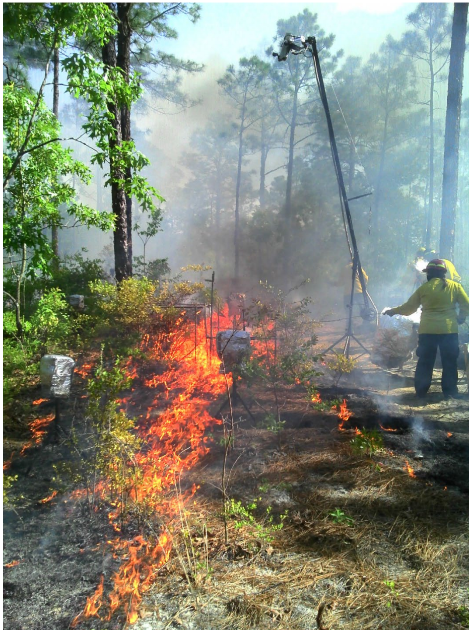
Figure 25. Boom-mounted IR camera used to measure shrub leaf temperatures during prescribed burns at Ft. Jackson, SC.
