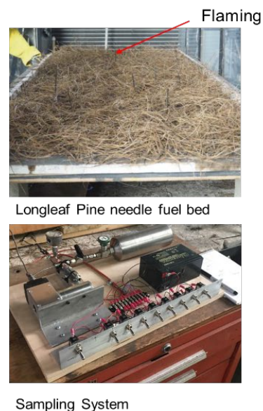
Figure 14. Setup of wind tunnel canister sample points.
