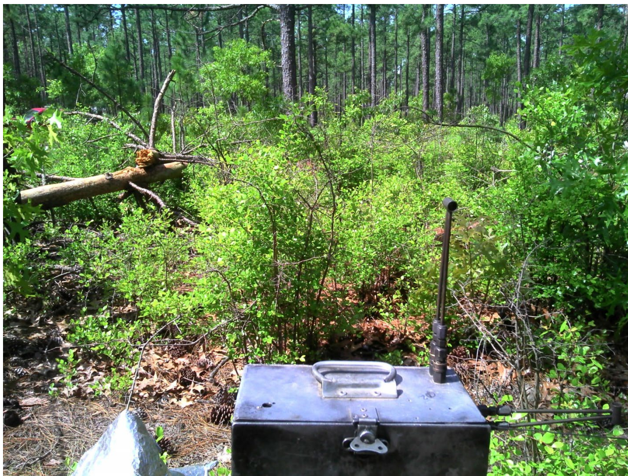
Figure 72. Fuel loading in plot 16D6. A peak total heat flux of 12.4 \text{ kW m}^{-2} was registered along with a peak air temperature of 631 \text{ }^{\circ}\text{C} and peak horizontal wind speeds of 4 \text{ m s}^{-1} .
