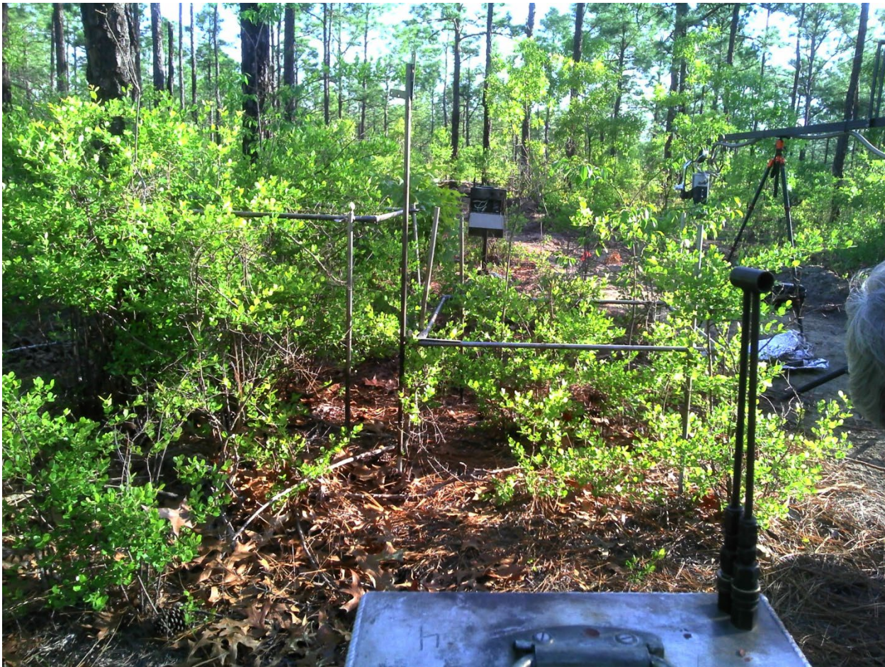
Figure 70. Instrumentation set up to monitor fire behavior in plot 16D5 reference plots.
