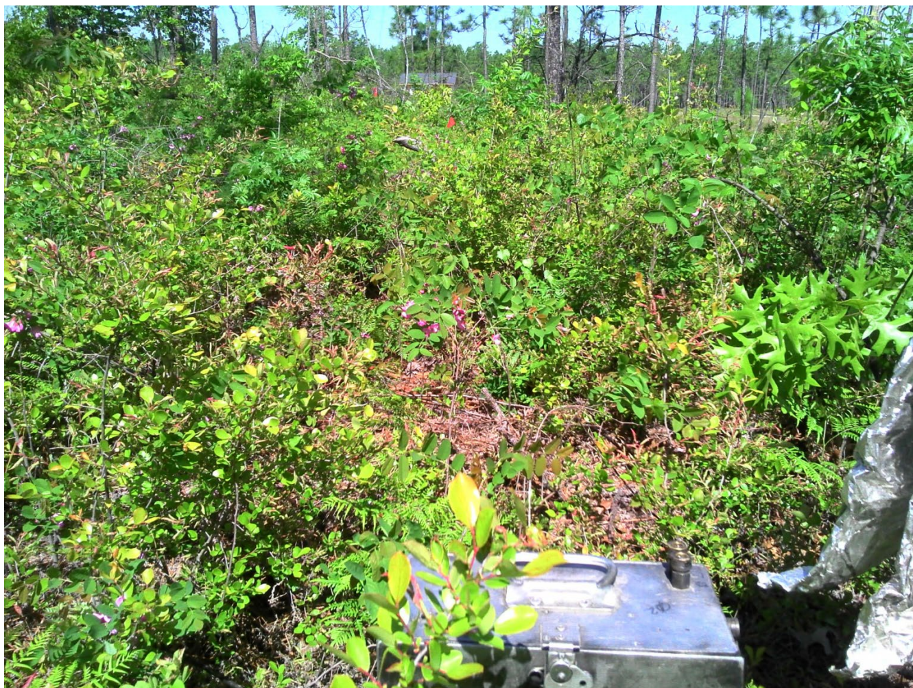
Figure 65. Fuel loading on plot 24Bs. A peak total heat flux of 30\text{kW m}^{-2} was registered for this burn along with a peak air temperature of 1042\text{ }^{\circ}\text{C} and a peak horizontal wind speed of 4\text{m s}^{-1} .
