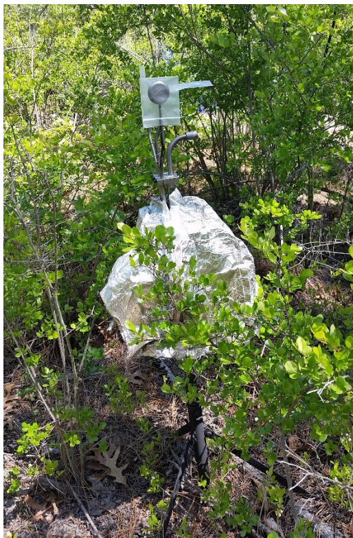
Figure 81. New heat flux package consisting of radiometer, a disk anemometer and thermocouples deployed in experimental prescribed burns in longleaf pine at Ft. Jackson, SC.
