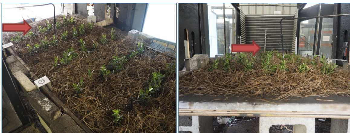
Figure 17. Fuel bed composed of longleaf pine needles and Lyonia lucida plants. Sample probe to collect pyrolysis gases for the Bruker Tensor 37 is indicated by the arrow.
