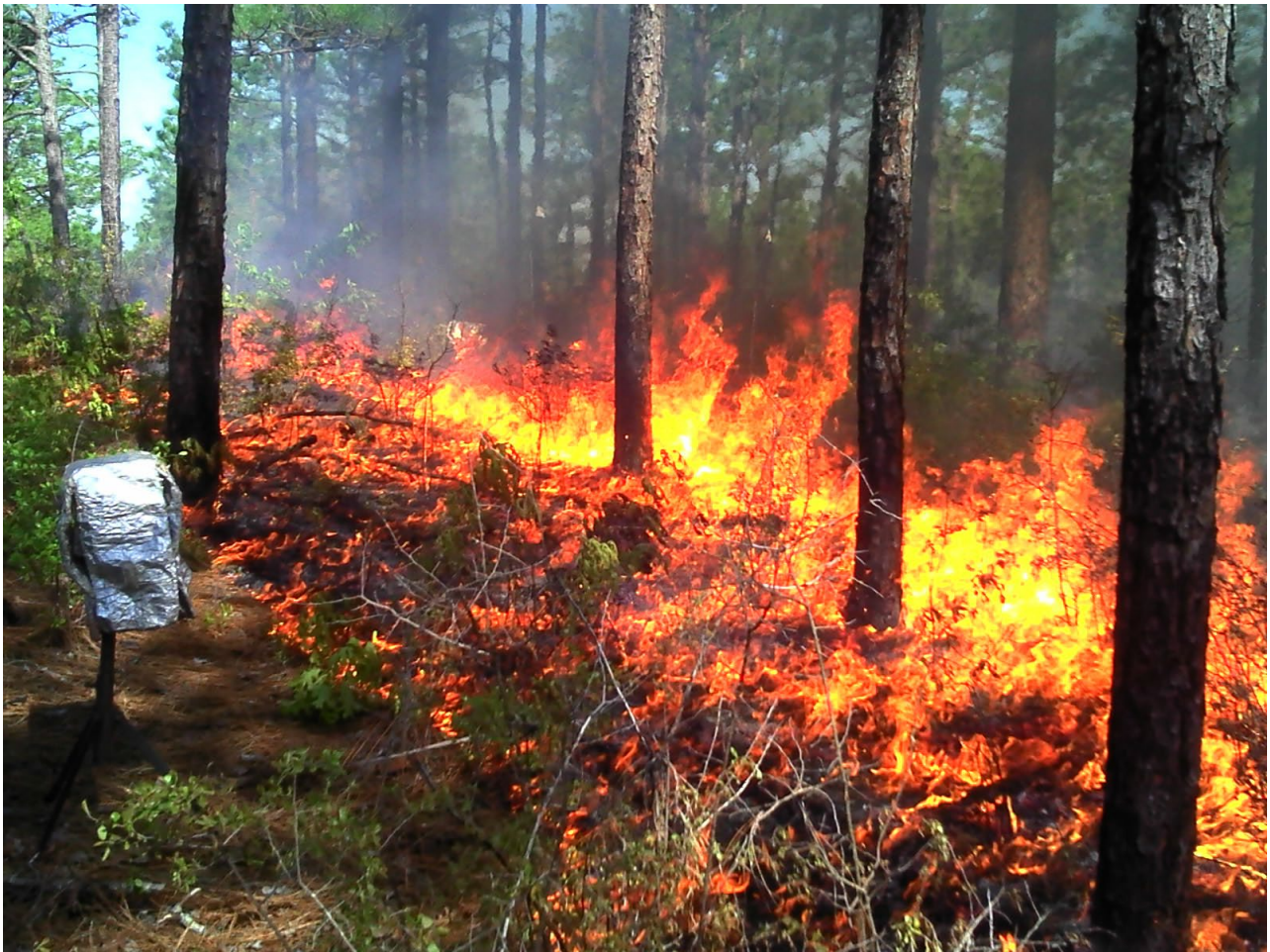
Figure 67. Fire behavior in 24As where a peak total heat flux value of 17.5 \text{ kW m}^{-2} was registered along with a peak air temperature of 954 \text{ }^{\circ}\text{C} and peak wind speed of 4.5 \text{ m s}^{-1} .
