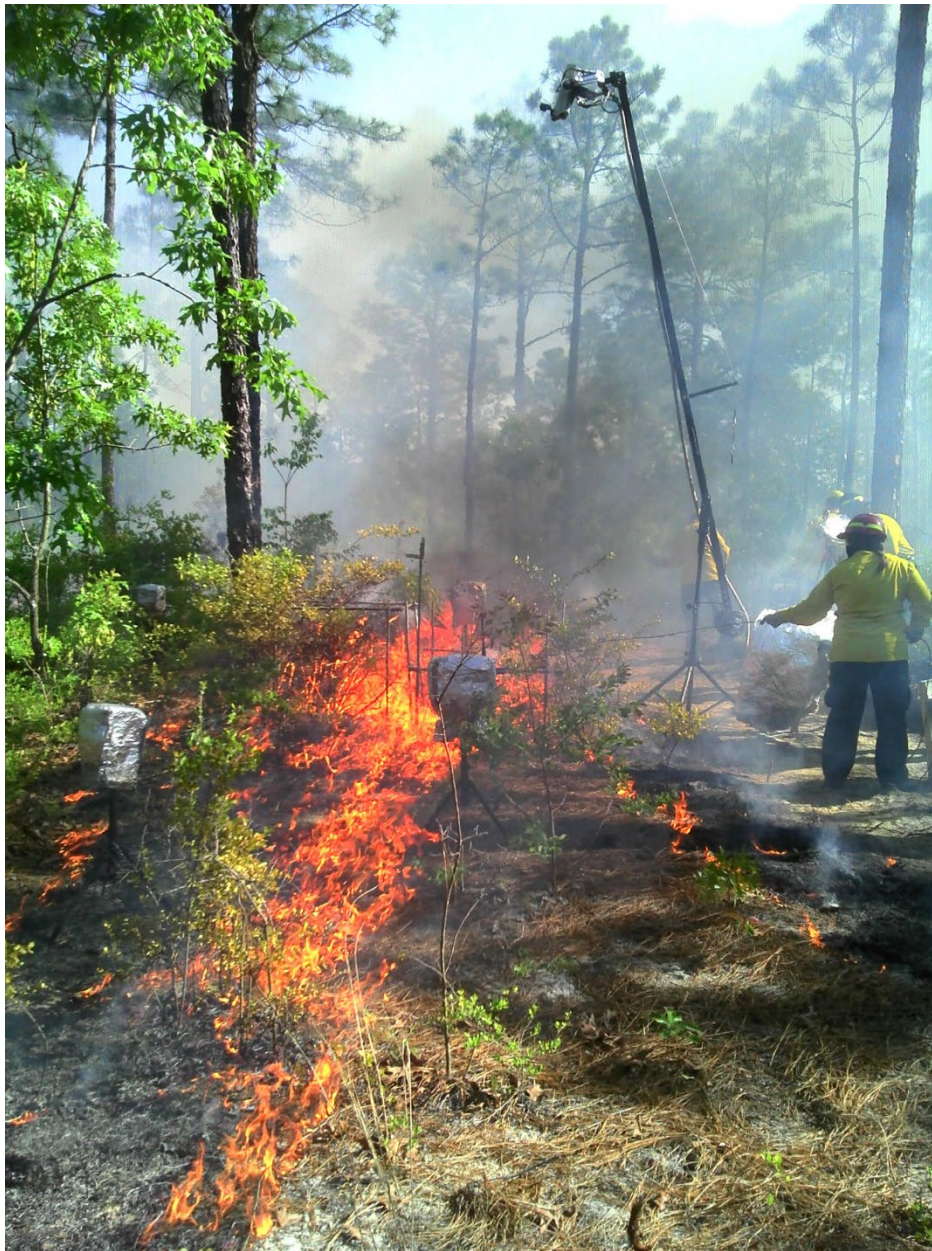
Figure 71. Fire behavior in plot 16D5 reference plots. A peak total heat flux of 10.9\text{kW m}^{-2} was registered for burn 5 along with a peak air temperature of 511\text{ }^{\circ}\text{C} , peak horizontal wind speed of 3.8\text{m s}^{-1} .
