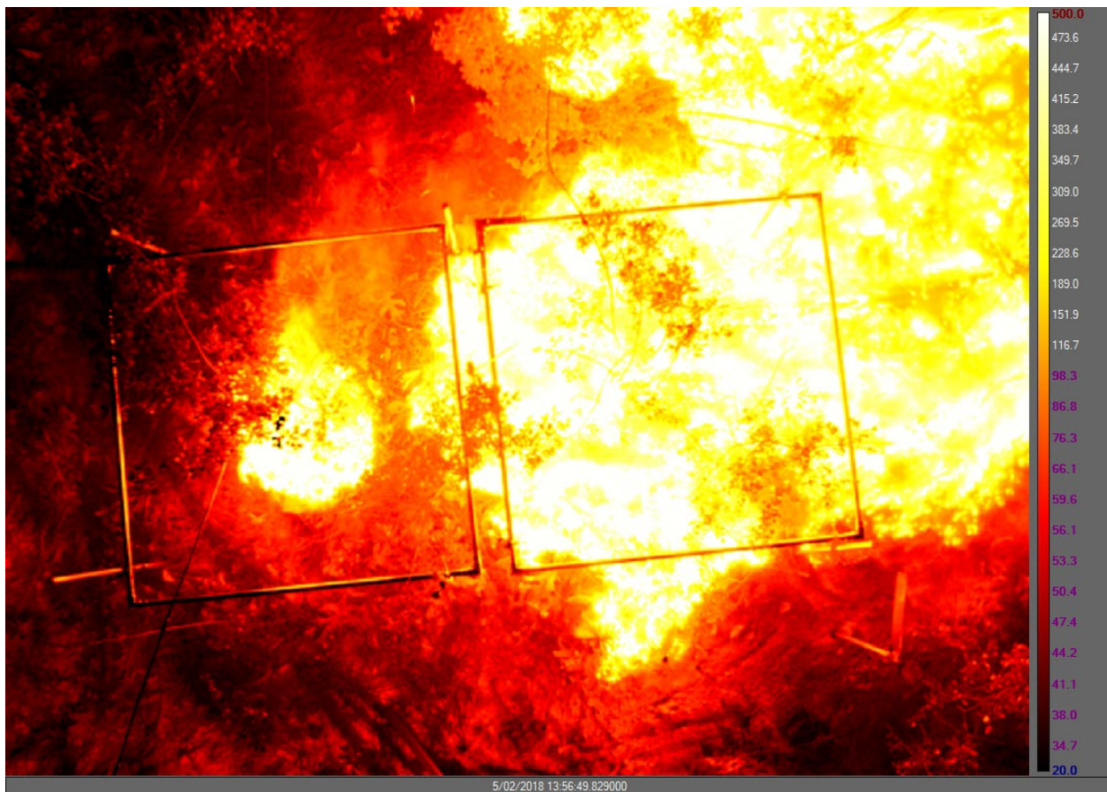
Figure 90. Example thermal image of plot 24A. The gas sampling wand is visible in the lower left.
