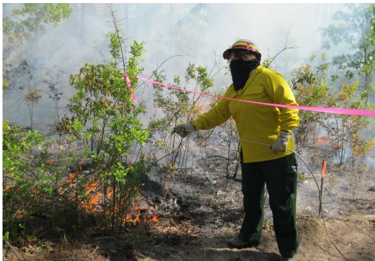
Figure 18. Gathering pyrolysis phase gas samples using an extractive wand coupled to a pump and gas canister (not seen) during prescribed burns at Ft. Jackson, SC, May 2018.
