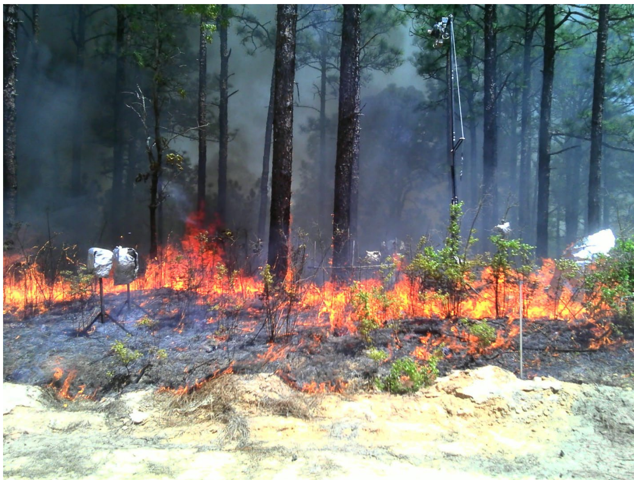
Figure 69. Fire behavior in the reference plots of plot 24At. Instruments registered a peak total heat flux of 19.3 \text{ kW m}^{-2} , a peak air temperature of 714 \text{ }^{\circ}\text{C} , and a peak horizontal wind speed of 3.6 \text{ m s}^{-1} .
