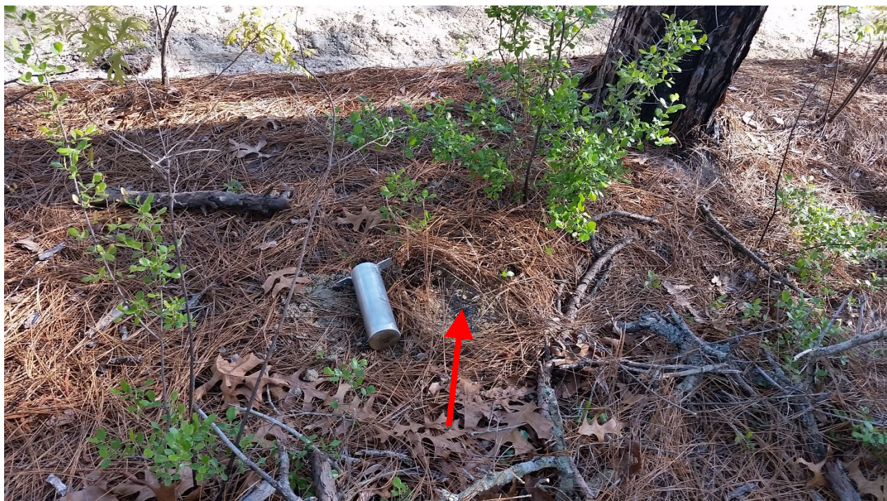
Figure 82. Flame ionization detector used to estimate flame residence time buried in longleaf pine forest floor at Ft. Jackson, SC. Red arrow indicates detector.
