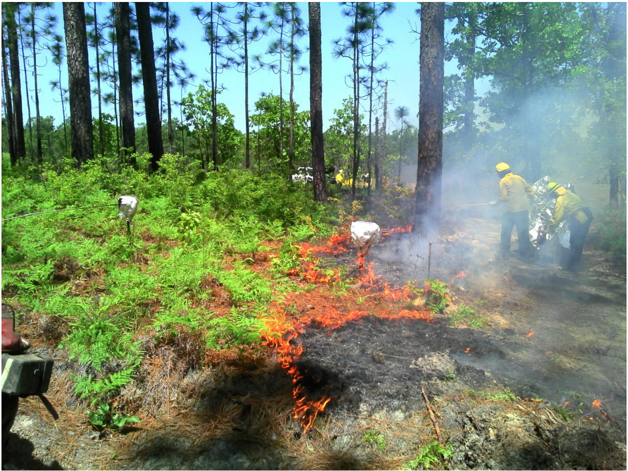
Figure 64. Fire behavior package 6 during burn in 24Bt. This package saw a peak total heat flux of 10.9 \text{ kW m}^{-2} , peak air temperature of 423^{\circ}\text{C} , and registered a peak wind speed of 3 \text{ m s}^{-1} .
